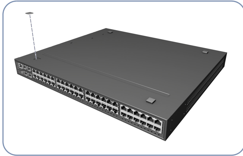
Figure 10: Attaching the Adhesive Feet
